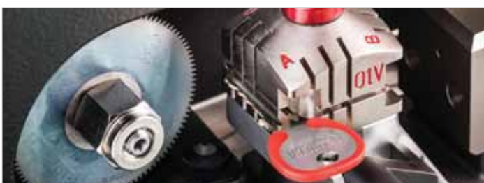
Flat and cruciform key cutting
