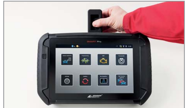
Expansion port and slot for Smart Aerial
